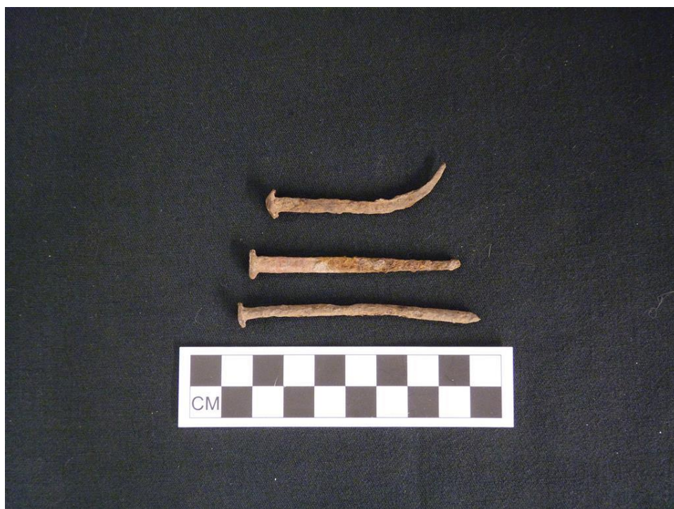
Image 16: Nails (top to bottom): wrought, machine cut, and wire.
